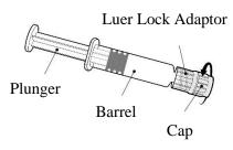
Hold the syringe by the barrel, not by the plunger.
