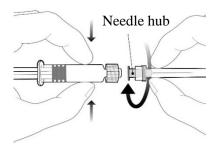
To attach the needle, connect the hub to the Luer Lock Adaptor and rotate a quarter turn clockwise until you feel it lock.
